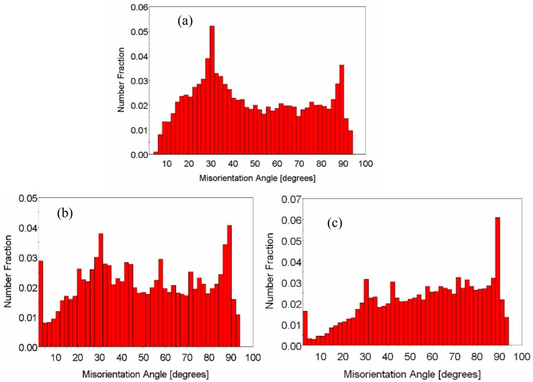
Fig.4 Grain boundary misorientations in the present alloys after CEC 7 pass at 225 °C, (a) AZ31 (b) AZ31-1Si and (c) AZ91.
