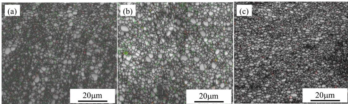
Fig.2 Grain structure maps viewed in the longitudinal section (SEM-EBSD) after CEC 7 passes at 225°C, (a) AZ31, (b) AZ31-1Si and (c) AZ91.
