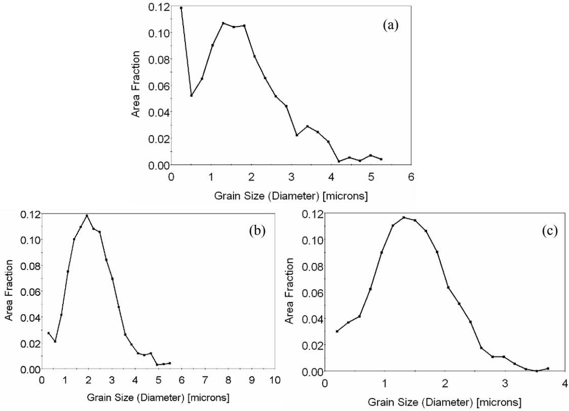
Fig.3. Grain size area fractions in the present alloys after CEC 7 passes at 225°C, (a) AZ31 (b) AZ31-1Si and (c) AZ91.
