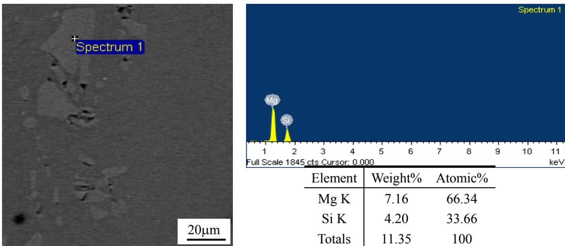
Fig.1  $Mg_2Si$  phase in extruded AZ31-1Si and the corresponding EDAX analysis.
