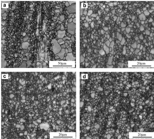
**Figure 1.** Grain boundaries map (SEM-EBSD) of as-extruded and alloys processed by CEC at 573 K: (a) as-extruded; (b) CEC 1 pass; (c) CEC 3 passes; (d) CEC 7 passes.
