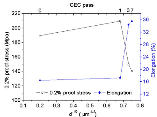
**Figure 6.** Measured 0.2% proof stress and elongation as a function of  $d^{-1/2}$ .
