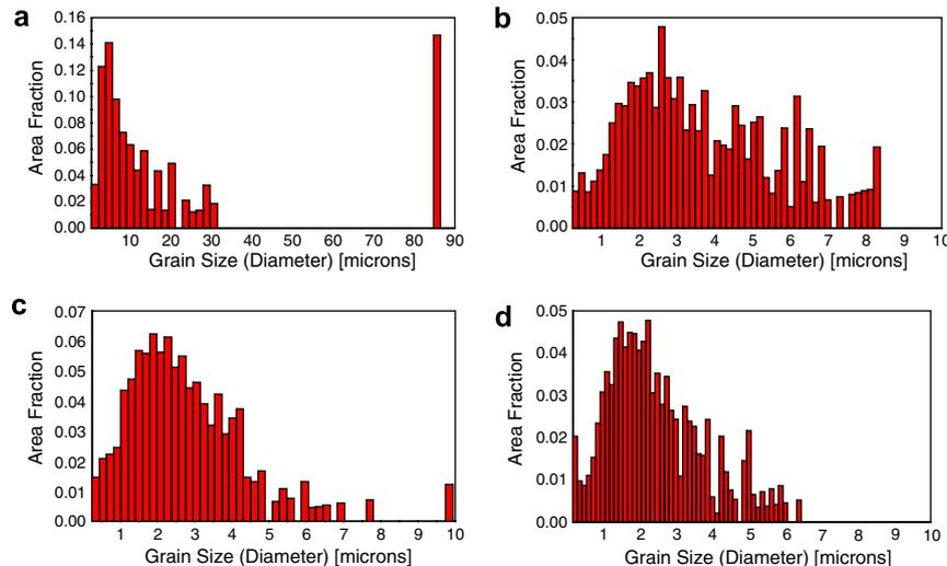
**Figure 2.** Grain-size distribution of as-extruded alloys and alloys processed by CEC at 573 K: (a) as-extruded; (b) CEC 1 pass; (c) CEC 3 passes; (d) CEC 7 passes.
