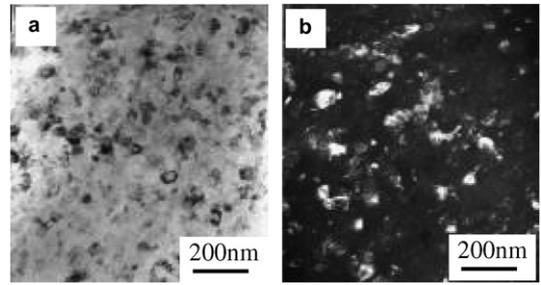
**Figure 3.** TEM micrographs of AZ31 alloy after CEC 7 passes and 573 K: (a) bright field; (b) corresponding dark field.
