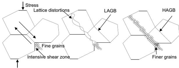
**Figure 5.** Schematic showing the grain refinement of magnesium alloys during CEC process (increasing strain accumulation going to the right).
