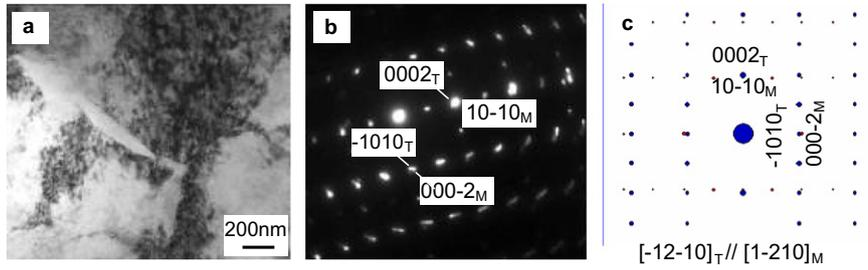
**Figure 4.** {10–12} twin in AZ31 alloy processed by CEC 3 passes and 573 K: (a) micrograph; (b) diffraction patterns of matrix and twin; (c) computer simulation of diffraction pattern of matrix and twin.
