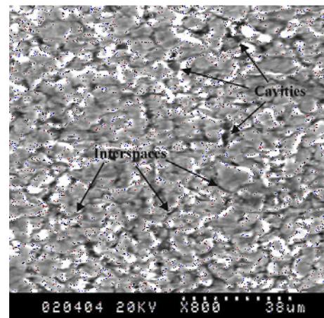
Fig. 5. Fracture surface of the rolled AZ91 after the best superplastic deformation.
