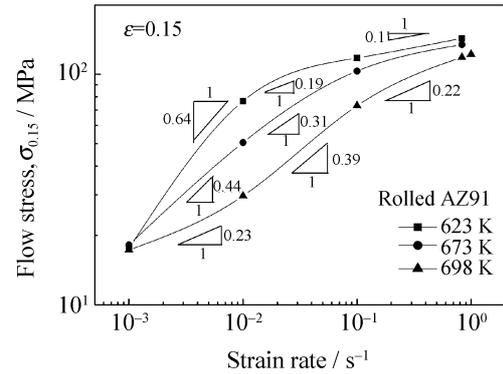
Fig. 2. Variation of flow stress as a function of strain rate.
