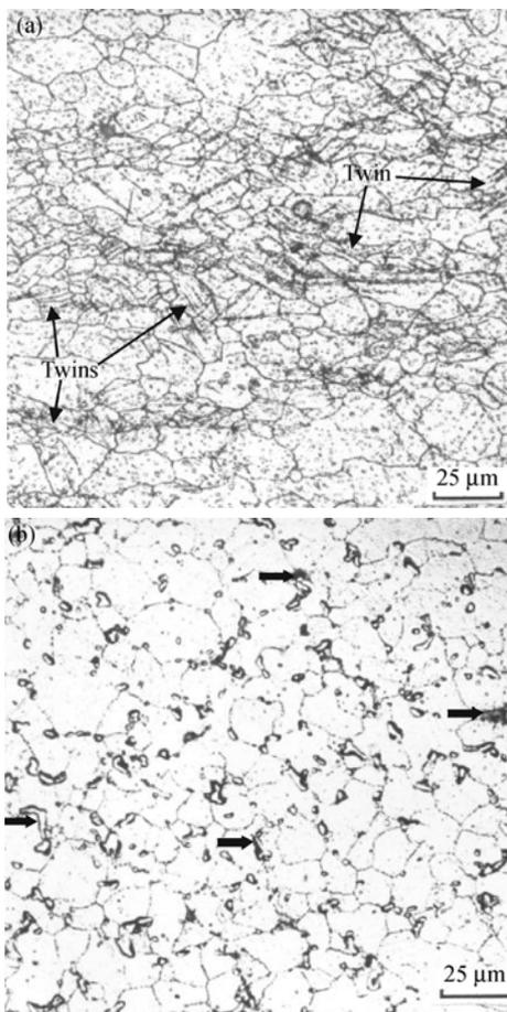
Fig. 4. Typical microstructures of the rolled AZ91 magnesium alloys before (a) and after (b) the tensile test with the maximum elongation of 455% (623 K,  $10^{-3} \text{ s}^{-1}$ ).
