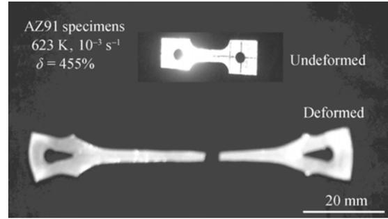
Fig. 1. Undeformed and fractured specimens of AZ91.
