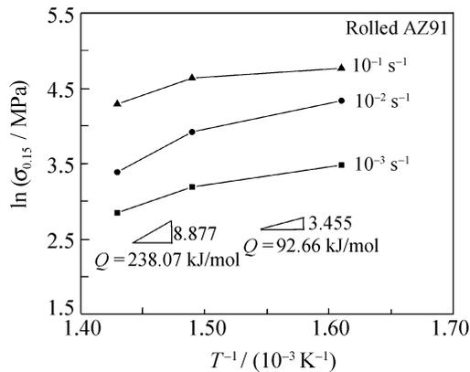
Fig. 3. Active energy curves of  $\ln \sigma_{0.15}$  versus  $1/T$  in the rolled AZ91 superplastic deformation.
