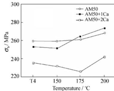
Fig. 3. Effect on aging treatment on the tensile strength of extruded AM50 + xCa alloys.
