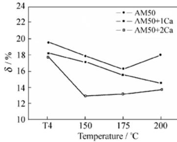
Fig. 4. Effect on aging treatment on the elongation of extruded AM50 + xCa alloys.
