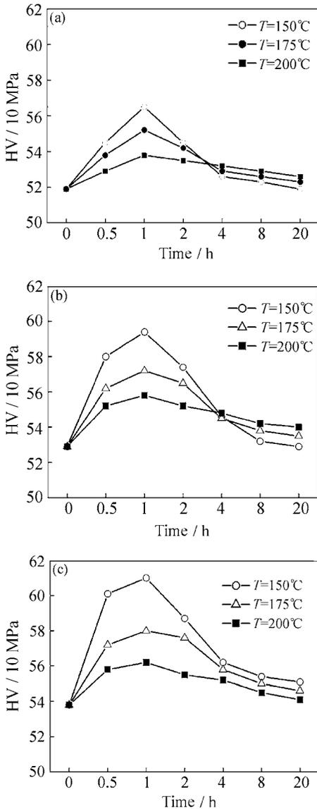
Fig. 2. Effect of aging treatment on the hardness of extruded AM50 + xCa magnesium alloys: (a) AM50; (b) AM50 + 1Ca; (c) AM50 + 2Ca.
