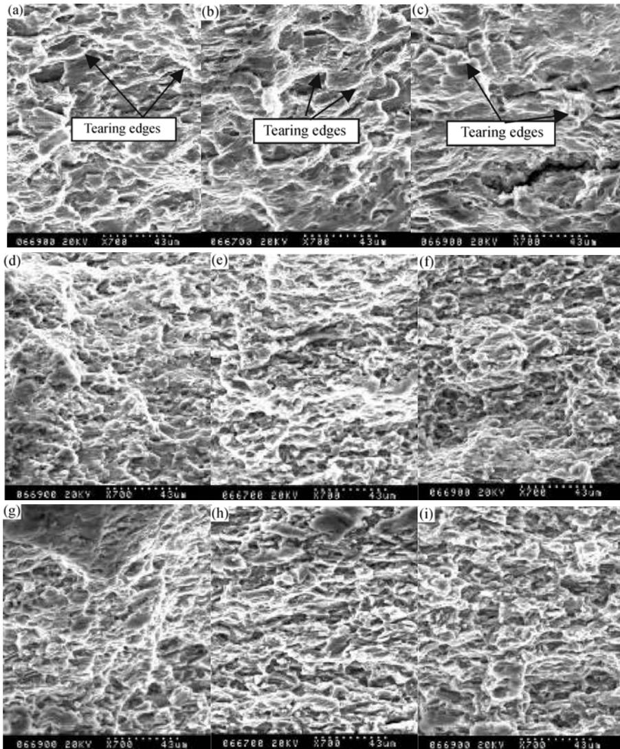
Fig. 5. Fracture surface SEM of extruded AM50 + xCa alloys after aging treatment: (a) AM50, T6 (150°C × 20 h); (b) AM50, T6 (175°C × 20 h); (c) AM50, T6 (200°C × 20 h); (d) AM50 + 1Ca, T6 (150°C × 20 h); (e) AM50 + 1Ca, T6 (175°C × 20 h); (f) AM50 + 1Ca, T6 (200°C × 20 h); (g) AM50 + 2Ca, T6 (150°C × 20 h); (h) AM50 + 2Ca, T6 (175°C × 20 h); (i) AM50 + 2Ca, T6 (200°C × 20 h).
