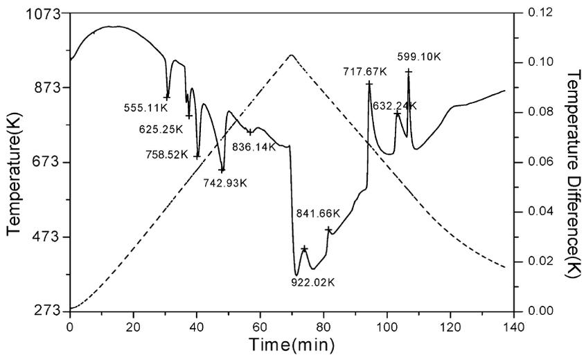
Fig. 5. DTA curve of Zn-27Al-6.3Mg-3.7Si alloy.
