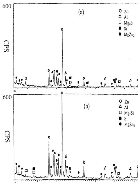
Fig. 2. X-ray diffractogram of (Mg<sub>2</sub>Si+Si)/AZ27 composites.
