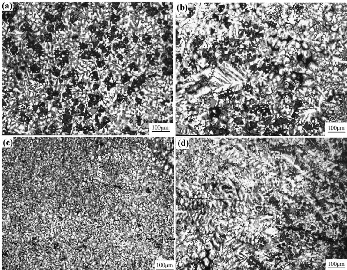
Fig. 1. Microstructure of  $(Mg_2Si + Si)/ZA27$  composites ( $T_m = 200\text{ }^\circ\text{C}$ ,  $n = 1000\text{ rpm}$ ). (a) Inner layer, (b) transitional layer, (c) middle layer, (d) outer layer.
