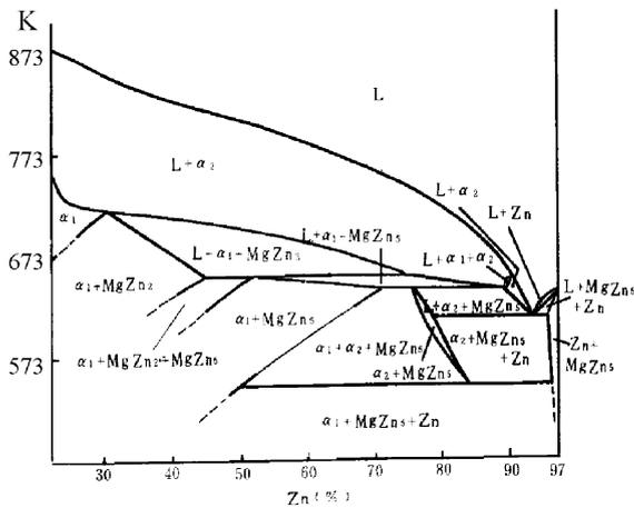
Fig. 6. The vertical projection of Zn–Al–3%Mg alloy.
