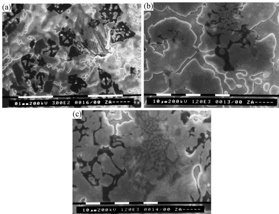
Fig. 3. SEMs of ( $Mg_2Si$ +Si)/ZA27 composite. (a) Inner layer, (b) and (c) outer layer.
