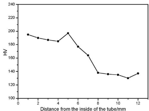
Fig. 8. Hardness distribution of composites.
