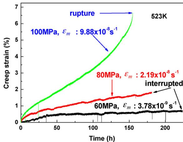
Fig. 9. Creep curves of the as-extruded Mg-4Y-4Sm-0.5Zr alloy at 523 K and at different stresses from 60 MPa to 100 MPa.
