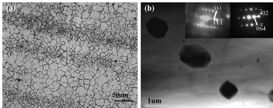
Fig. 2. Microstructure of the as-extruded Mg-4Y-4Sm-0.5Zr alloy. (a) Optical micrograph. (b) TEM image of the precipitates in the as-extruded alloy. The inserts show the diffraction patterns corresponding to the precipitates.
