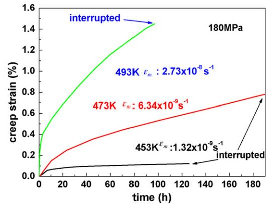
Fig. 7. Creep curves of the as-extruded Mg-4Y-4Sm-0.5Zr alloy at 180 MPa and at different temperatures from 453 K to 493 K.
