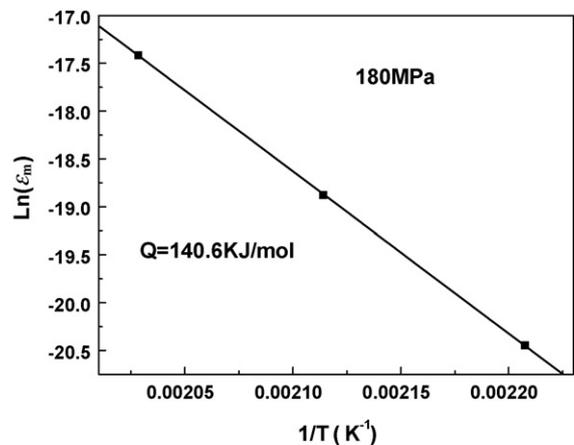
Fig. 8.  $\ln(\dot{\epsilon})-(1/T)$  curve of the as-extruded Mg-4Y-4Sm-0.5Zr alloy crept at 180 MPa.
