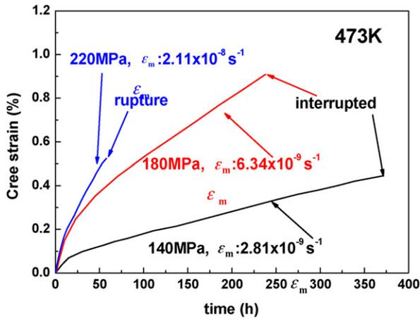
Fig. 5. Creep curves of the as-extruded Mg-4Y-4Sm-0.5Zr alloy at 473 K and at different stresses from 140 MPa to 220 MPa.
