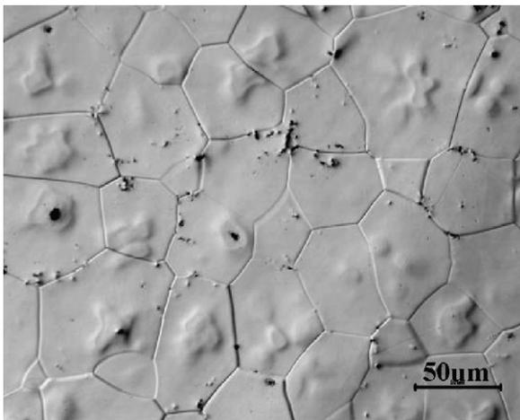
Fig. 1. Optical micrograph of the homogenized Mg-4Y-4Sm-0.5Zr alloy.
