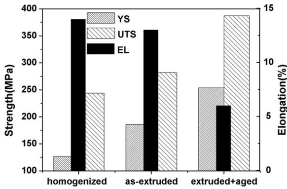
Fig. 4. Tensile properties of the Mg-4Y-4Sm-0.5Zr alloy in different states.
