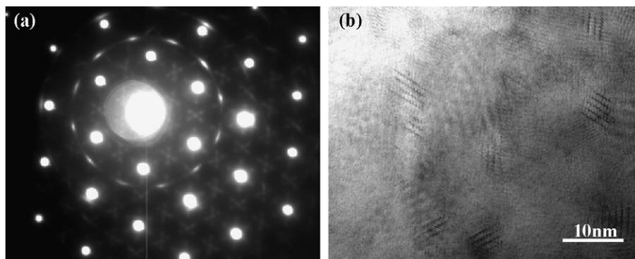
Fig. 3. SAED pattern and HRTEM image of precipitates within the grains in the extruded Mg-4Y-4Sm-0.5Zr alloy after ageing at 473 K for 16 h, beam direction:  $[0001]_a$ : (a) SAED pattern; (b) HRTEM image.
