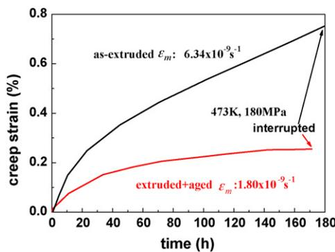
Fig. 10. Creep curves of the as-extruded and extruded-plus-aged Mg-4Y-4Sm-0.5Zr alloy at 473 K and 180 MPa.
