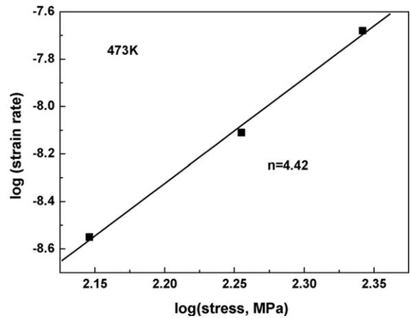
Fig. 6.  $\log(\text{strain rate})-\log(\text{stress})$  curve of the as-extruded Mg-4Y-4Sm-0.5Zr alloy crept at 473 K.
