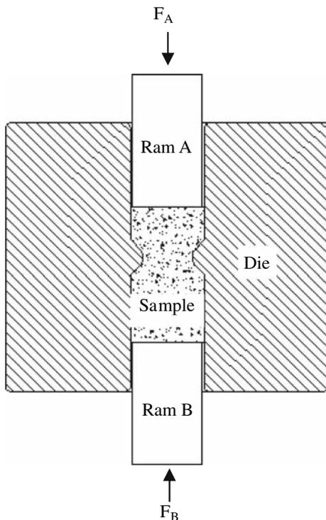
**Fig. 1** A schematic drawing of CEC method
