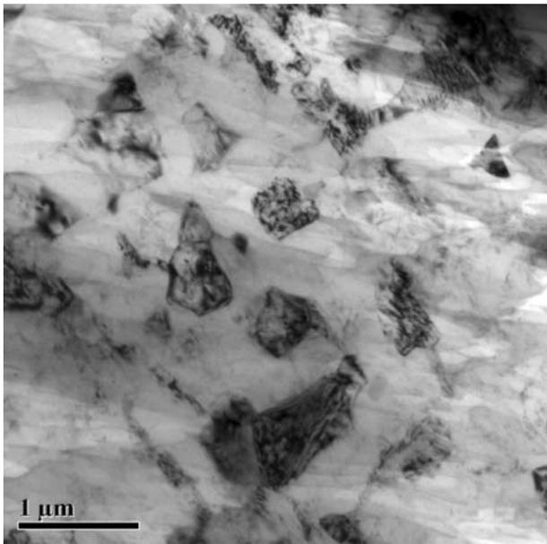
**Fig. 3** TEM bright-field micrograph from the longitudinal section of AZ31 Mg alloy processed by the CEC method after 6 passes
