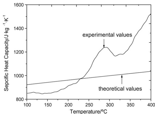
**Fig. 3.** Comparison of the measured and calculated curves of specific heat capacity.
