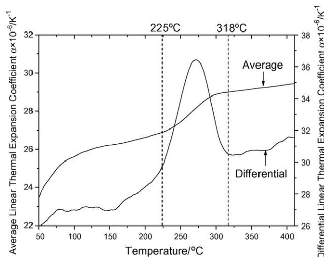
Fig. 5. Linear thermal expansion coefficient of WGZ115 alloy.
