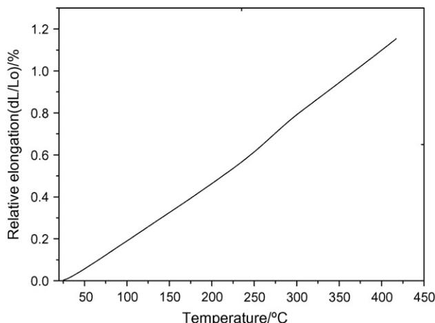
**Fig. 4.** Relative elongation of WGZ115 alloy (25–400 °C).
