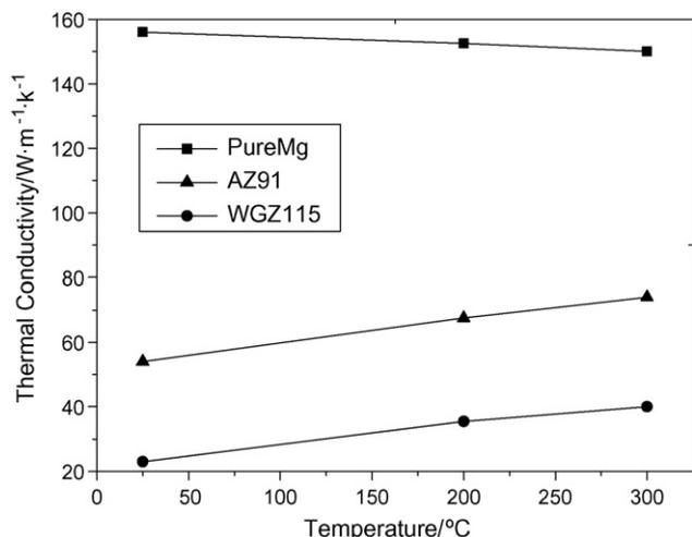
Fig. 7. Thermal conductivity of WGZ115 alloy, pure Mg and AZ91.
