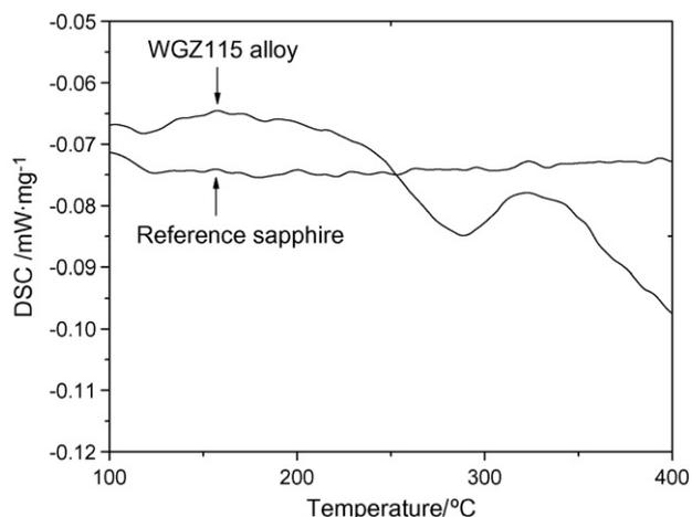
**Fig. 2.** Curves of DSC of WGZ115 alloy and reference sapphire (100–400 °C).
