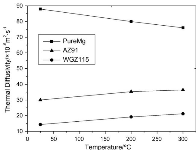
Fig. 6. Thermal diffusivity of WGZ115 alloy, pure Mg and AZ91.
