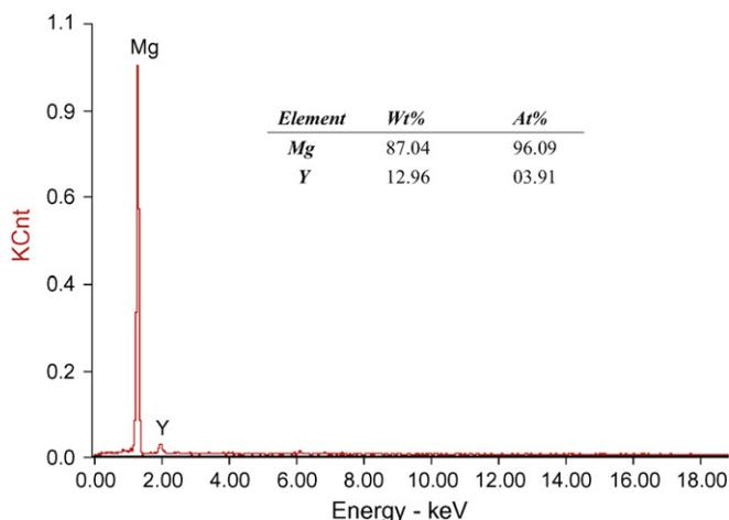
Fig. 8. EDX analysis of the WGZ115 alloy matrix phase.
